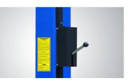
Single-Point Safety Release The Single-point safety release makes it easy for the operator to unlock both columns locks from one column, and more reliable !
