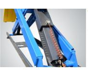
$\triangleleft$ Electro-air mechanical safety lock is more convenient and safe.
