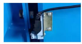
The safety stop device at the height of 300mm with tone alarm for safety.
