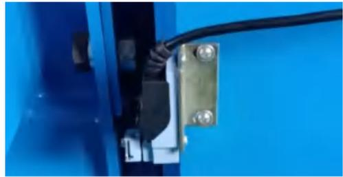
▲ The safety stop device at the height of 300mm with tone alarm for safety.
