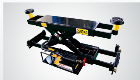
▲ Optional Rolling Jacks J6H: manual hydraulic type 2,800KG. J6A: pneumatic hydraulic type 2,800KG.
